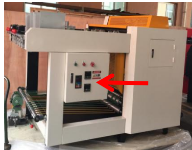
Electrical box and electrical parts
