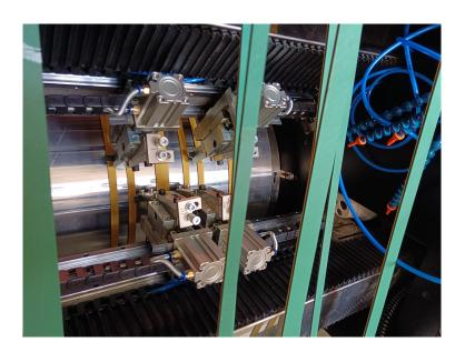
Servo System to find the knife, save a lot of knife adjusting time
