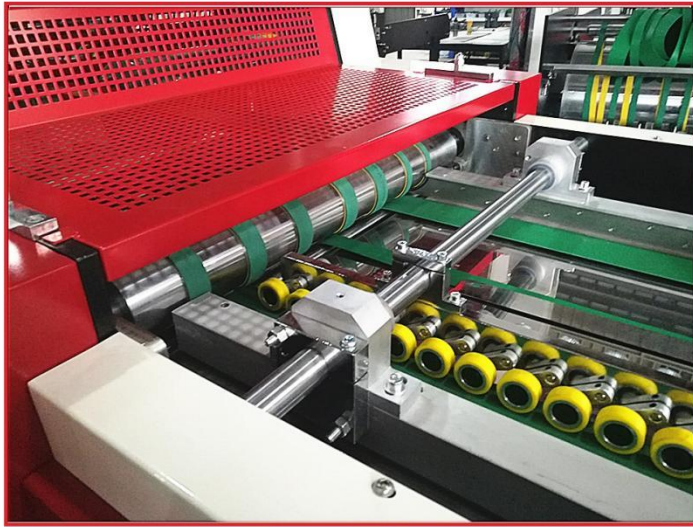
Auto Feeding With Anti-friction Belt
