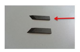
Blade Life: usually the blade can work 10000pcs after the first time sharping. And 1pc blade can been sharpened about 25-30 times under good using.
