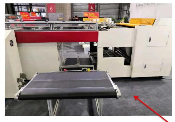
Automatic collector belt for the final production:
