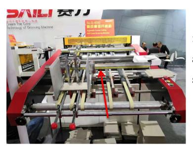
To put the pile of material on the feeding section, and the belts with the aligning system will automatically send the cardboard into grooving area. The final product will be conveyed out to the collecting table.
