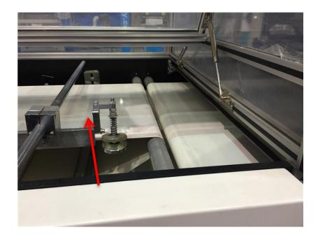
90 Automatic change the board direction for the 2<sup>nd</sup> step corner cutting and 2<sup>nd</sup> step grooving. www.sai-li.com
