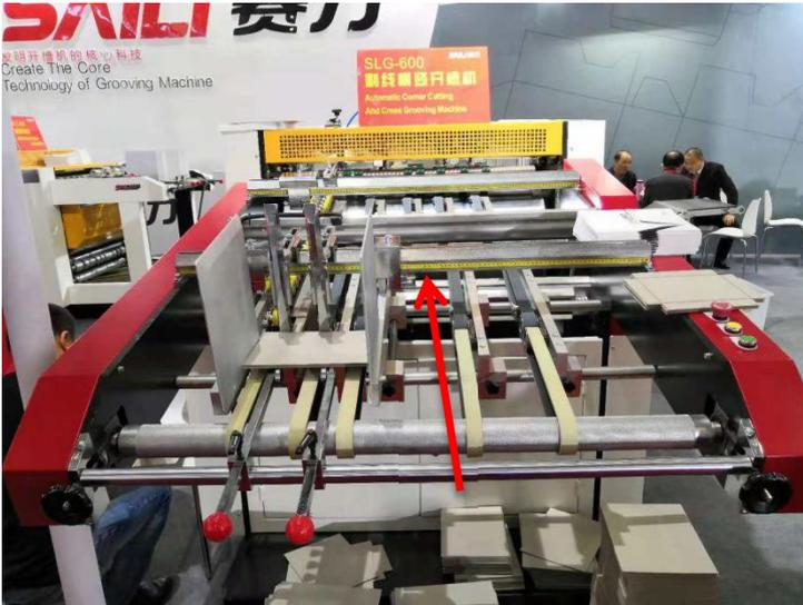
To put the pile of material on the feeding section, and the belts with the aligning system will automatically send the cardboard into grooving area. The final product will be conveyed out to the collecting table.
