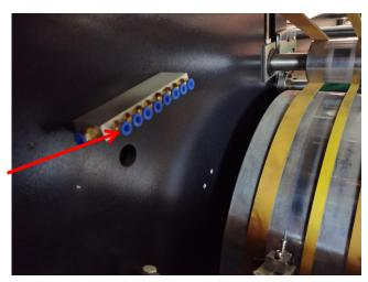
Automatic Waste Blowing Tubes are assembled in machine.
