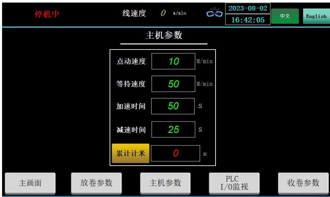
**Jog speed:** Press the external jog button to set the jog speed of the host in meters per minute. External jog button, which is the main engine jog function in the shutdown state and the constant speed function in the running state.
