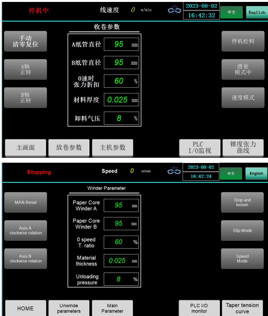
A Paper Tube Diameter: Set the diameter of the paper tube used for the A winding shaft.
