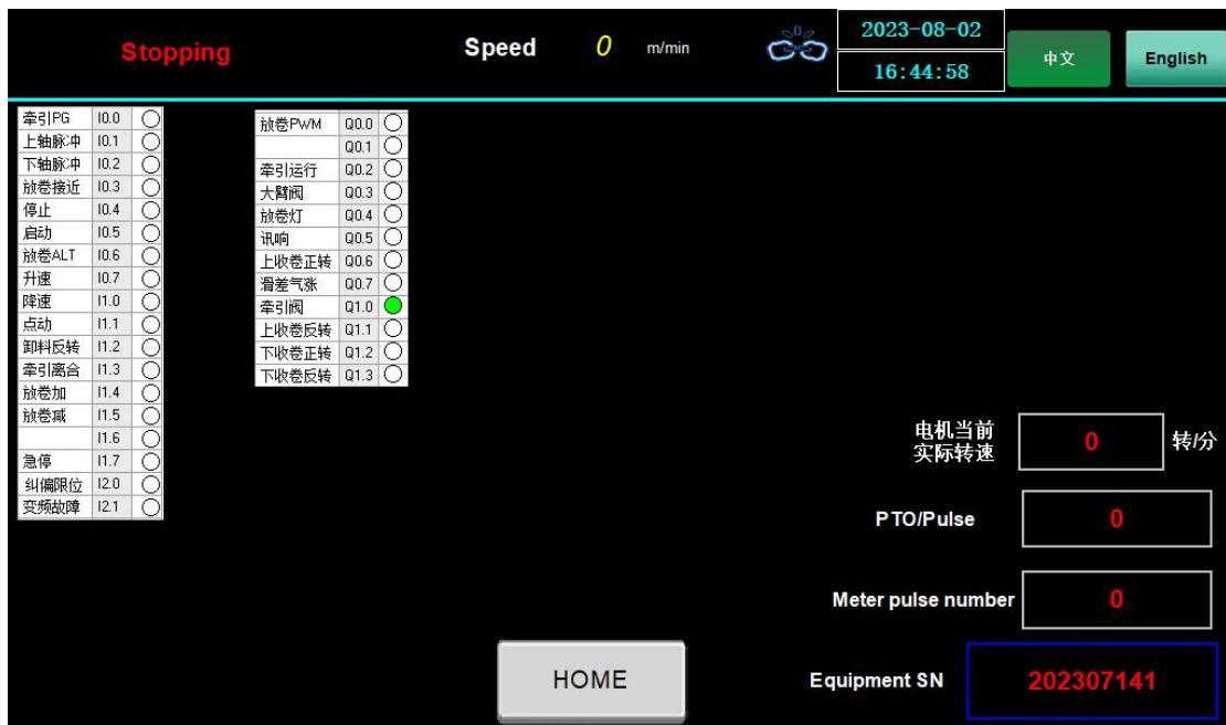
Monitor the input and output actions of the PLC, and the corresponding working lights will light up.
